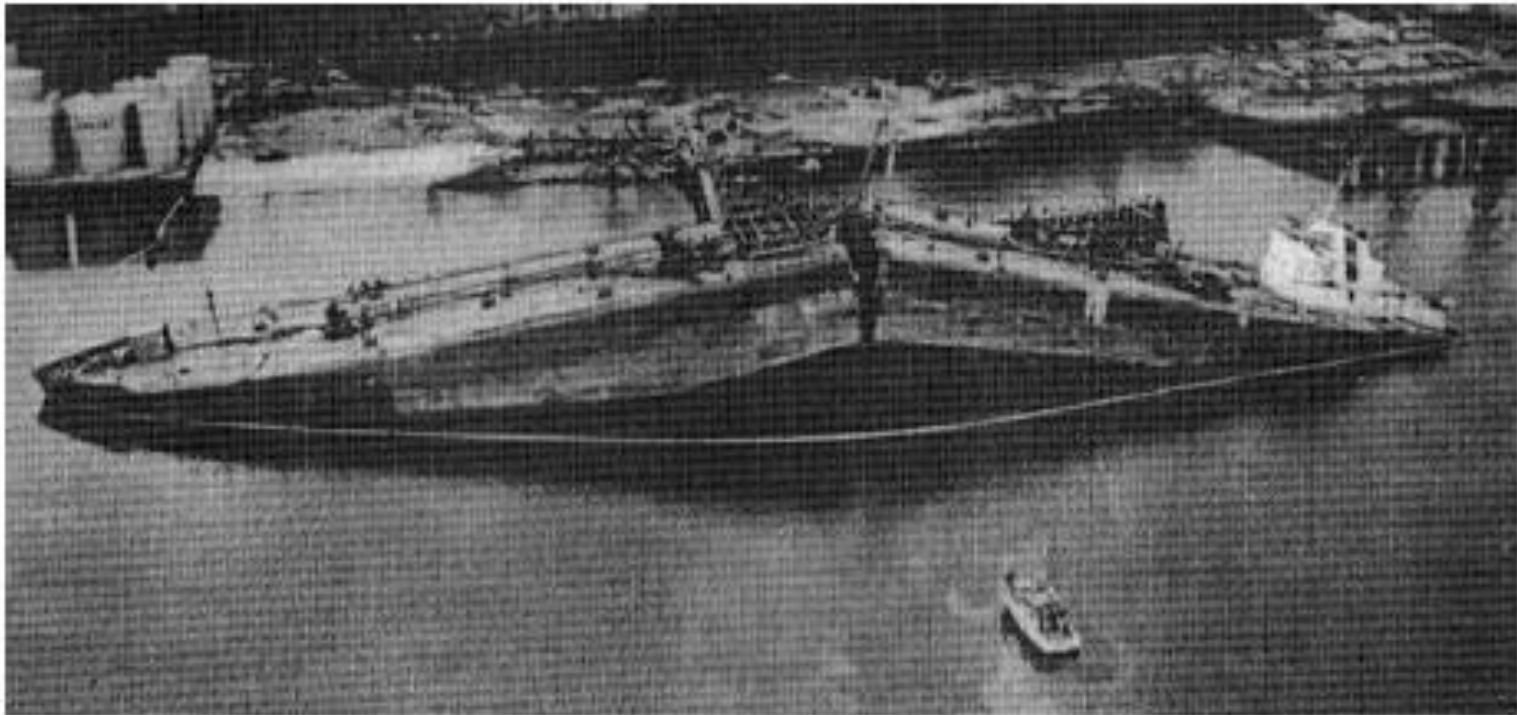
Fig. An oil barge that fractured in a brittle manner by crack propagation around its girth (The New York Times)
